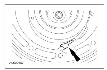
67. CAUTION: To avoid a "fall-out" condition of the strut from the screw during assembly and function, the small "U" shape notch should be toward the band/case side and the large "U" shape notch toward the main control side.
